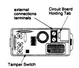
Note: To guard against static, place the circuit board in the sensor cover before continuing.
